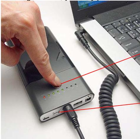
Press the capacity button to see the remaining capacity.
