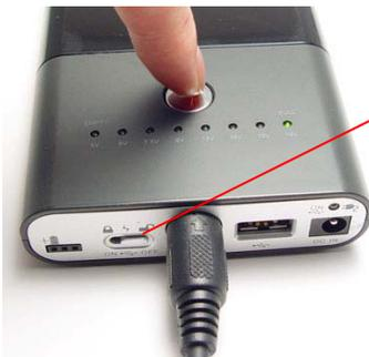
Switch to the right
