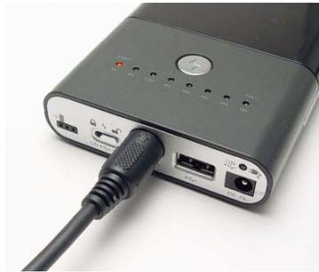
2. Select a suitable DB plug and connect it to the Power Output Cable. At this point, the 5V LED indicator should light up, indicating normal output operation
